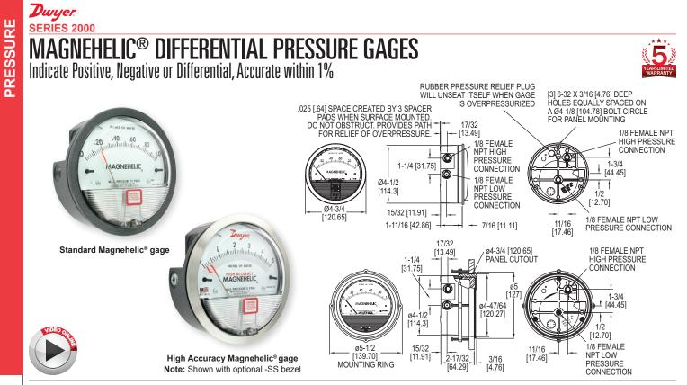
Select the Series 2000 Magnehelic® Differential Pressure Gages for a versatile low differential pressure gage with a wide choice of 81 models and 27 options to choose from. Using Dwyer's simple, frictionless Magnehelic® gage movement, it quickly indicates air or non-corrosive gas pressures--either positive, negative (vacuum) or differential. The design resists shock, vibration, over-pressures and is weatherproof to IP67.
